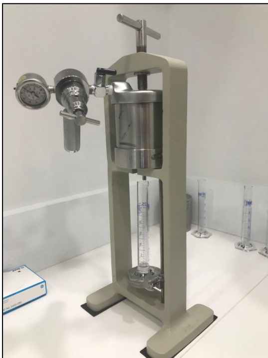
Laboratory filter press for measuring fluid loss of drilling fluids
